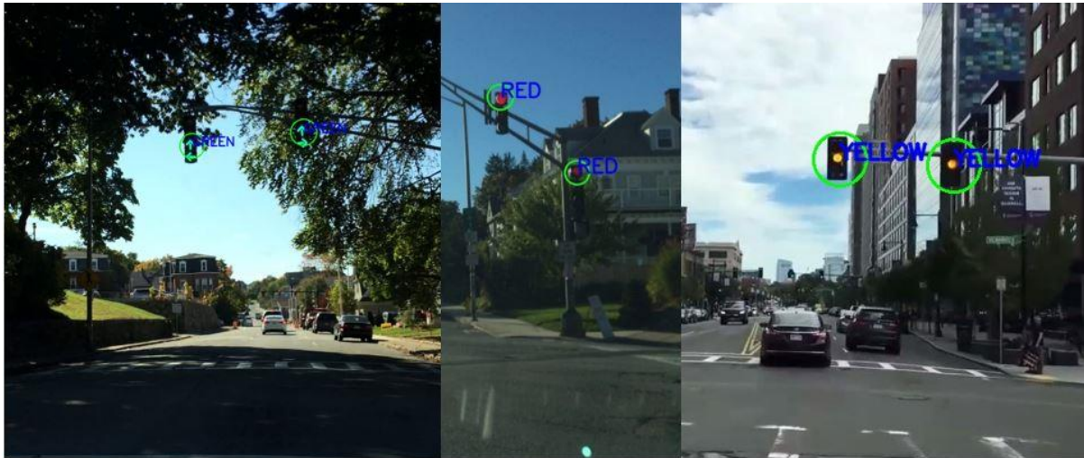
Fig 20: Final output of Hough Transform and Thresholding on HSV image algorithm
