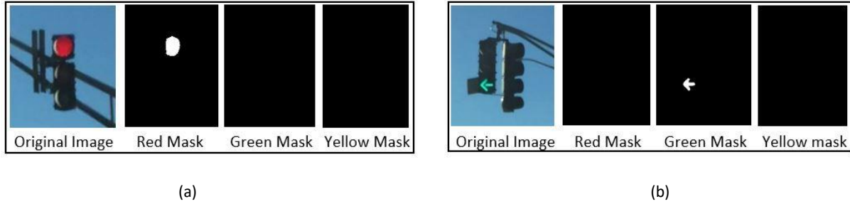
Fig 17. Binary mask for Red, Green and Yellow: (a) with Red signal as Input Image, (b) with green signal as Input Image
