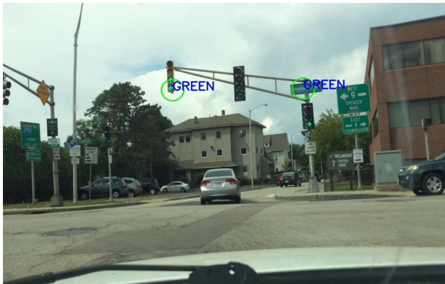
Fig 21: Case where Hough Transform and Thresholding on HSV image algorithm fails
