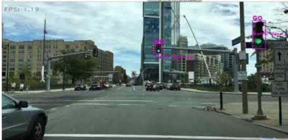
Fig 26. A still from the video of Appendix 6 where Yolov3 was applied on real-time video
