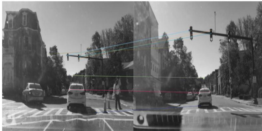
Fig 3: SIFT on two images of same scene but different perspective.
