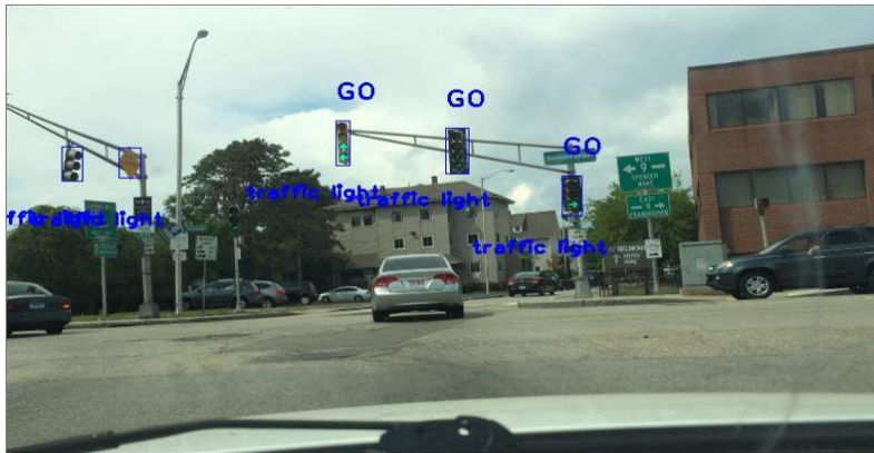
Fig 24: Applying YOLO and detecting the status of the signal
