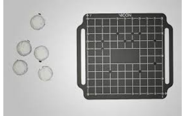
Fig. 5: Vicon rigid body markers and force plate
